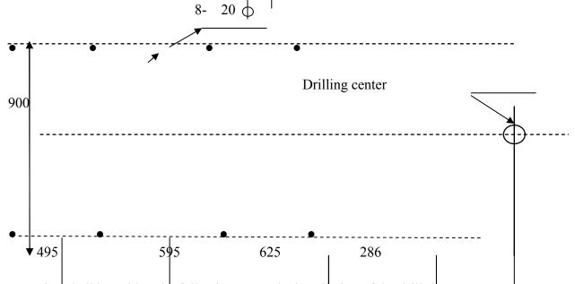
Attention shall be paid to the followings as to the installation of the drill rig: 1. Vertical shaft center, bore orifice and crown block pulley center of the drill rig shall be in the same line.
